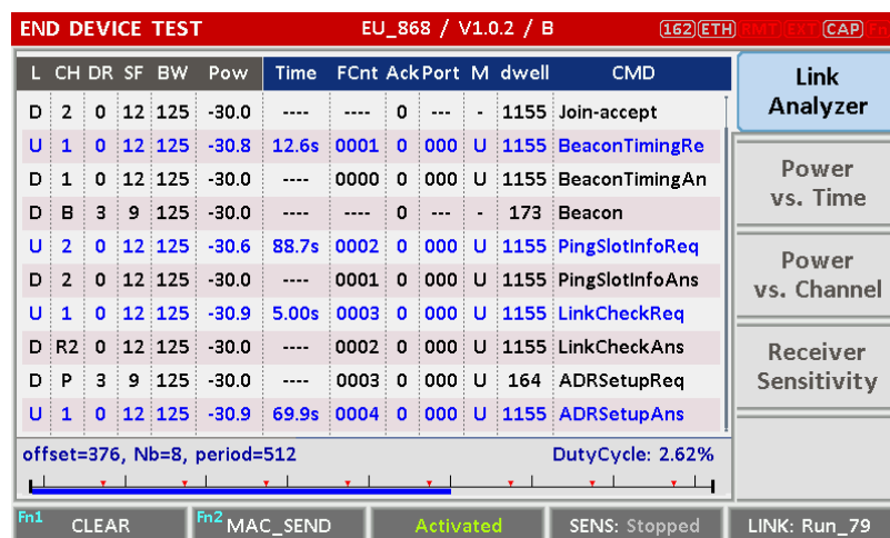
Fig 3.17 MAC command transmission through PING slot
